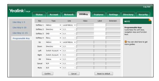
(Optional.) Enter a string that will appear on the LCD screen in the Label field.Label is configurable only when customizing SoftKey 1-4.
